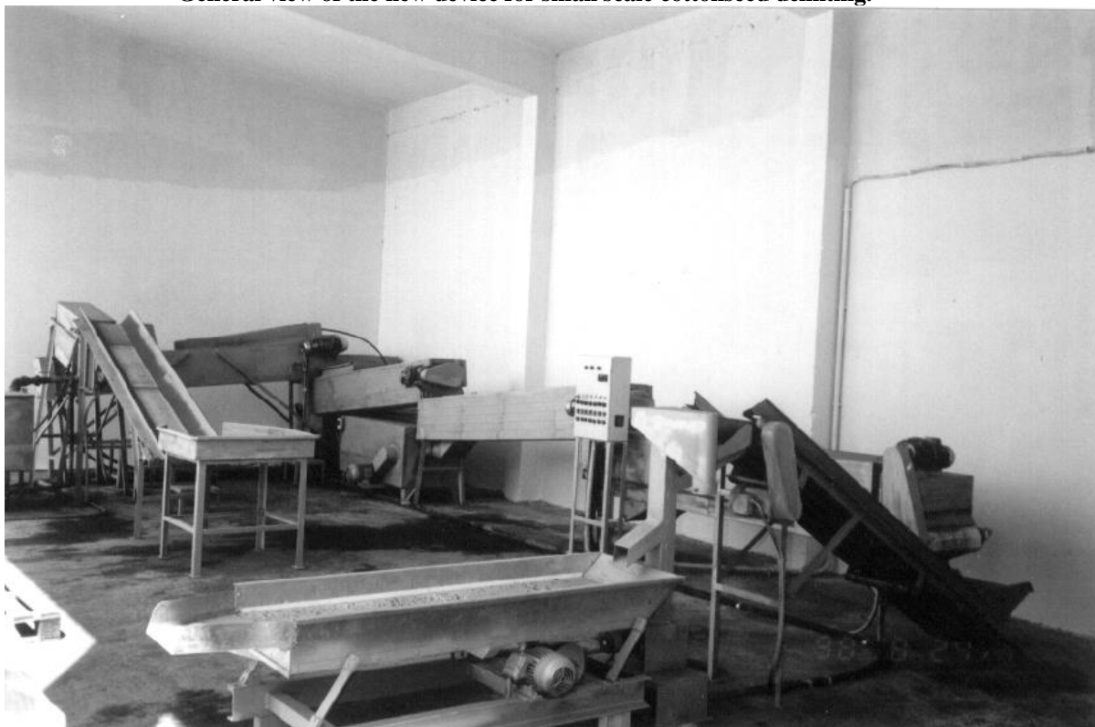
General view of the new device for small scale cottonseed delinting.
