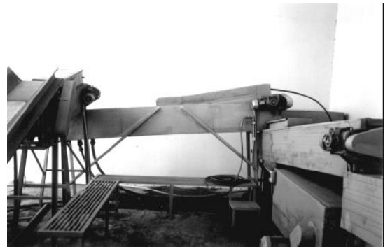
Picture 8. Seed cleaning and sieving system.
