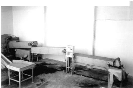
Picture 7. Seed drying system.
