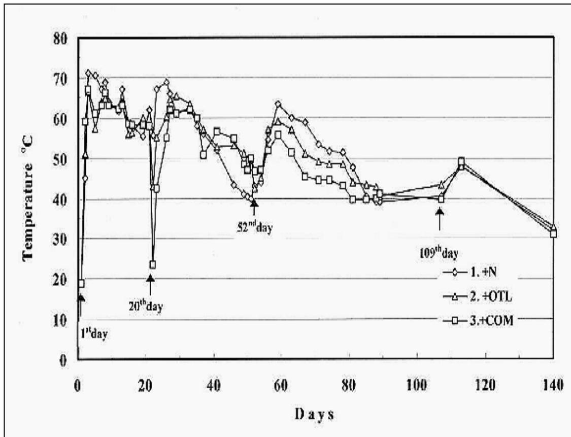
Figure 2. Variation of physical and chemical parameters with age in the piles. 1<sup>st</sup> pile: +N, with addition of NH<sub>4</sub>NO<sub>3</sub>, 2<sup>nd</sup> pile: +OTL, with addition of OTL, 3<sup>rd</sup> pile: +COM, with addition of mature compost from OTL.
