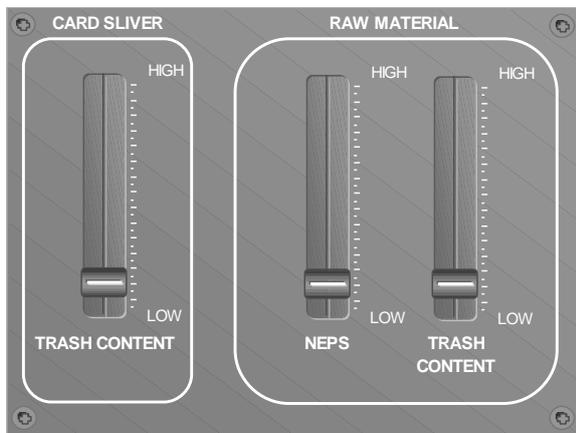
**Figure 8. Effect of raw material and mechanical processing on card sliver trash content.**
