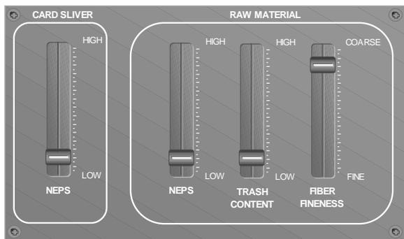
Figure 4. Effect of raw material and mechanical processing on neps in the card sliver.
