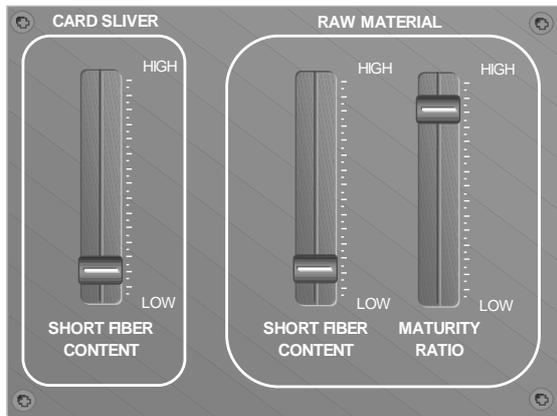
**Figure 12. Effect of raw material and mechanical processing on SFC of the card sliver.**
