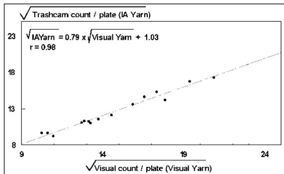
**Figure 7. Trashcam on yarn plate vs UT3 count open end spun 20 tex yarn.**
