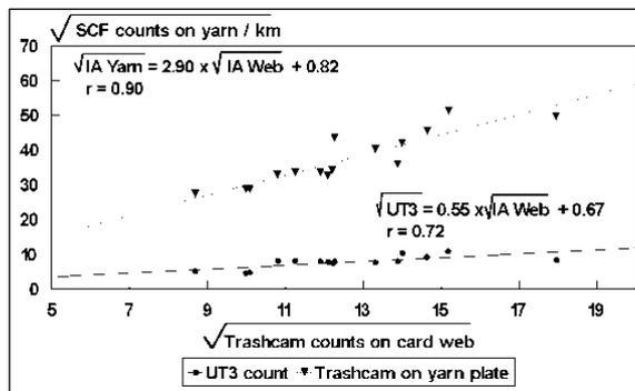
**Figure 5. Trashcam on yarn plate vs visual count on yarn plate; Open end spun 20 tex yarn.**
