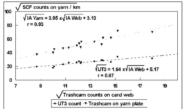
**Figure 4. Trashcam on yarn plate vs visual count on yarn plate ring spun 20 tex yarn.**
