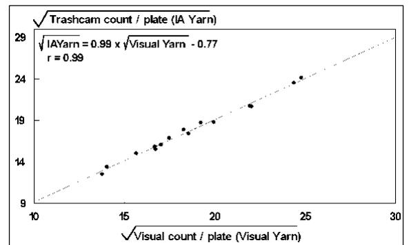
**Figure 6. Trashcam on yarn plate vs UT3 count ring spun 20 tex yarn.**
