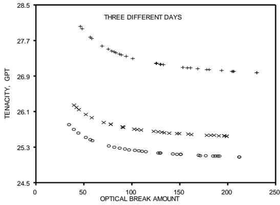
Figure 9. How RH% and breakage rate affect tenacity.
