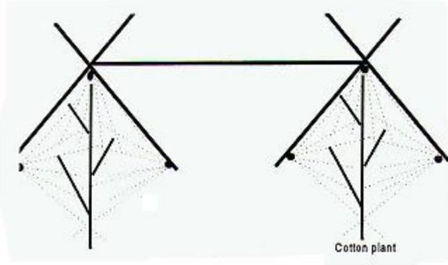
**Figure 2. Spray nozzle configuration, plants more than 400 mm tall, spray two half rows simultaneously with 6 nozzles per row**
