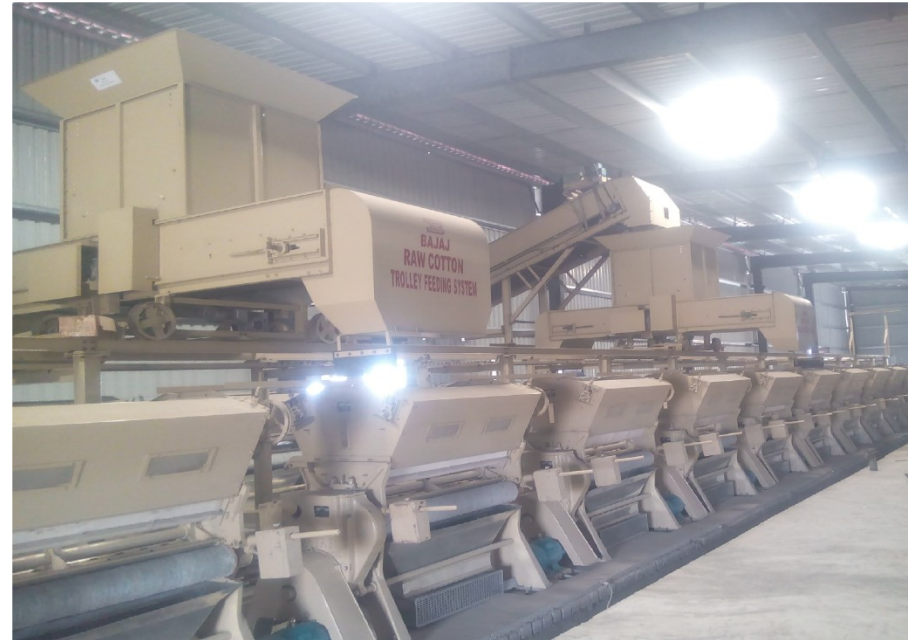
Seed Cotton Trolley Feeding System in Gin Hall
