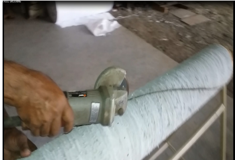
Leather Roll Groove cut by hand saw
