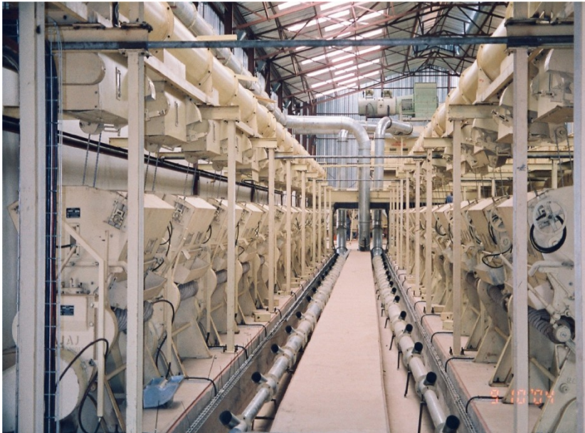
Intermediate Ducting arrangement for lint suction from Individual Double Roller Gin Machine
