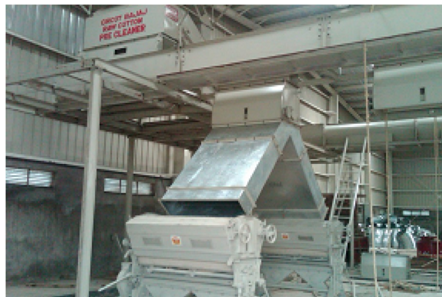
Central Distribution Screw Conveyor with Twin Feed Regulator
