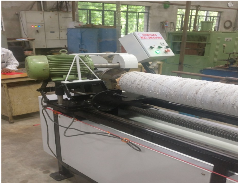
Automatic Leather Roll Grooving Machine
