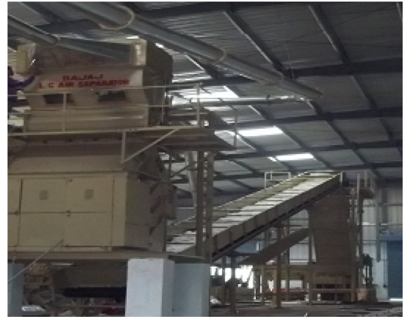
Lint Conveying by Belt to Press
