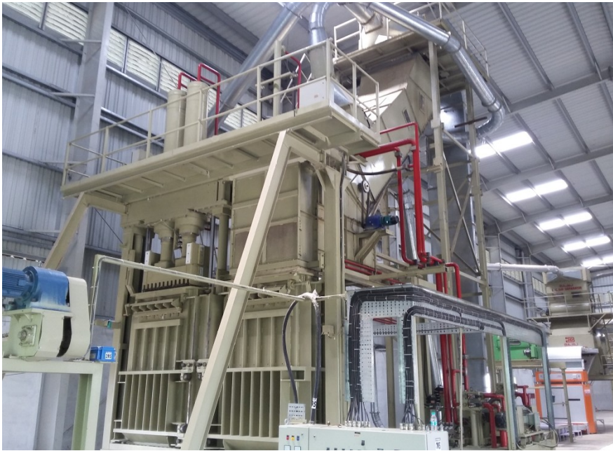
Lint Conveying by suction to Press
