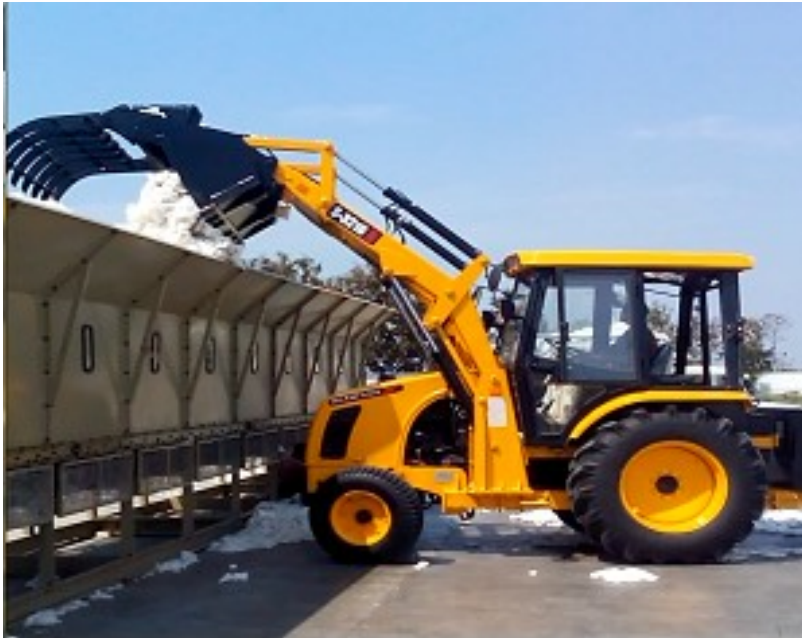
Seed Cotton Feeding by Tractor Attachment
