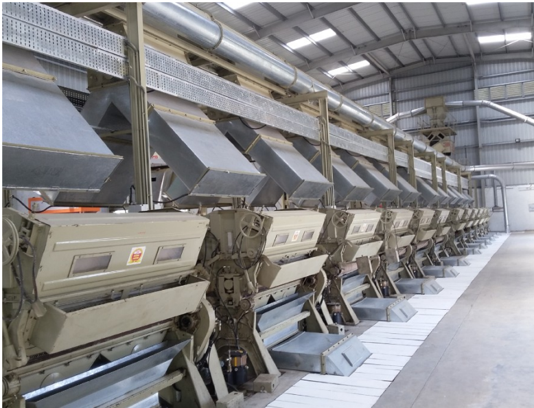
Lint Conveying by suction from each gin
