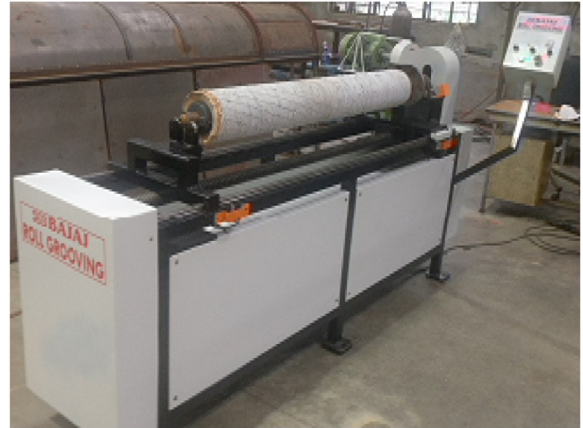
Automatic Leather Roll Grooving Machine
