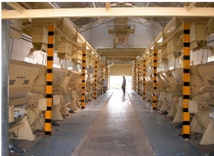
Individual Double Roller Gin Distribution Screw Conveyor with Single Feed Regulator
