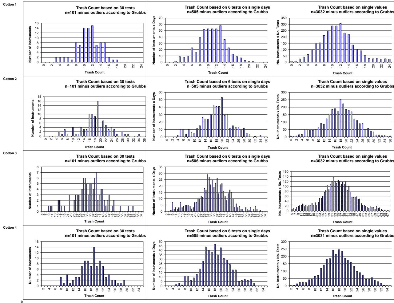
(Only results from instruments/days/single tests that are not regarded as outliers according to Grubbs' method)
