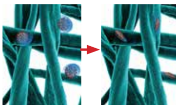
Schematic diagram to show how virion-aerosol droplets are absorbed and the virions desiccate and dry.
