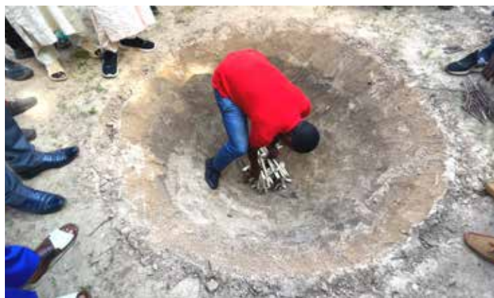
Figure-24. Preparing a chimney at the bottom of the pit and ignite it from the top.
