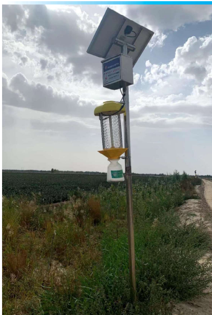
A solar-powered insect trap for analysing insects variety and quantity, in order to make reasonable and controlled chemical choices accordingly.
