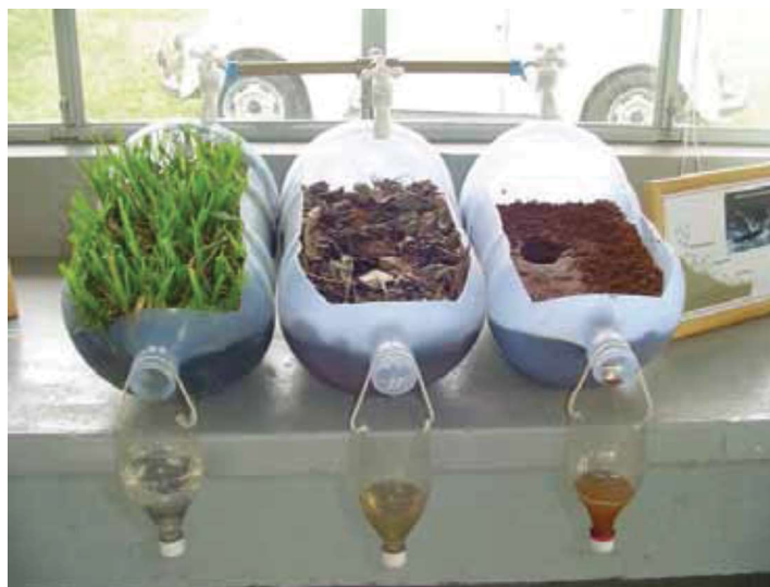
Effect of cover crops on soil erosion: Laboratory demonstration
