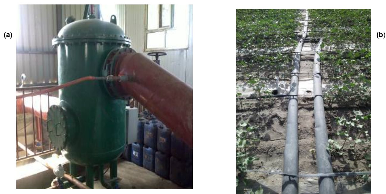
Fig. 4 Fertigation in drip irrigation under plastic mulching: (a) tank containing fertiliser for fertigation; (b) drip irrigation belt
