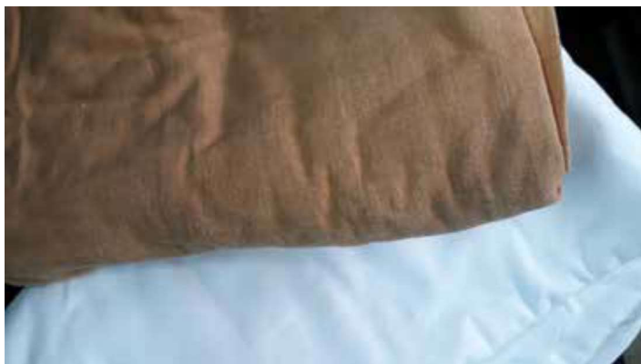
Figure 2. Cotton fabric treated with nano-silver (light brown above). The colour is due to the surface plasmon effect of nano-silver.
