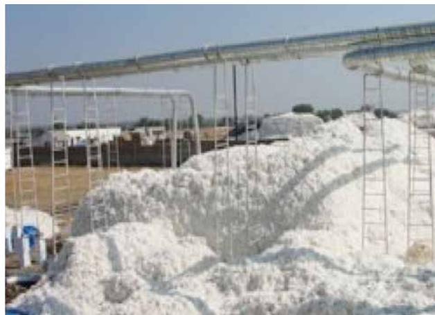
Figure 55. Seed cotton suction system
