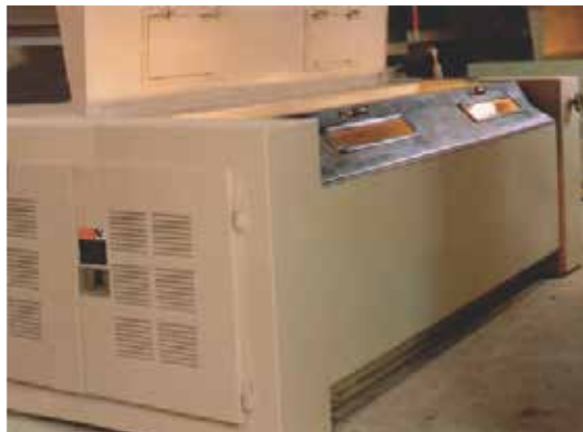
Figure 37. Hot air humidification system used for restoration of lint moisture
