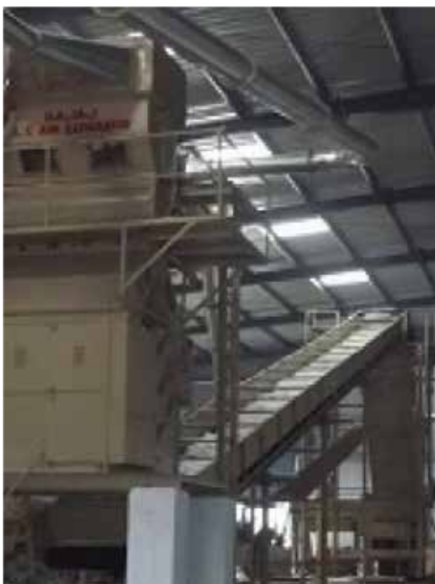
Figure 56. Lint conveying by belt
