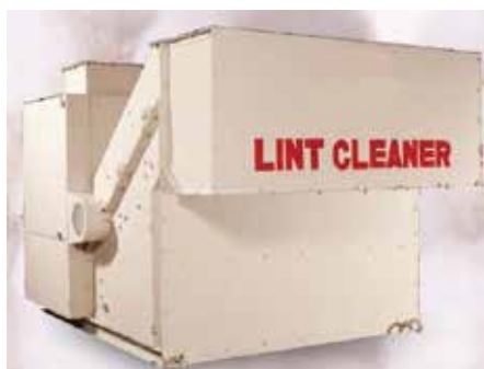
Figure 34. Spiked cylinder lint cleaner for handpicked cotton
