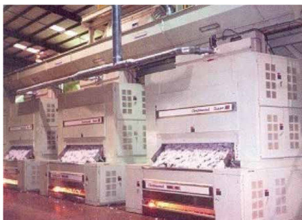
Figure 1. Saw gin machine
