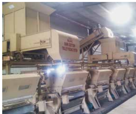
Figure 22. Seed-cotton dispenser with stone remover
