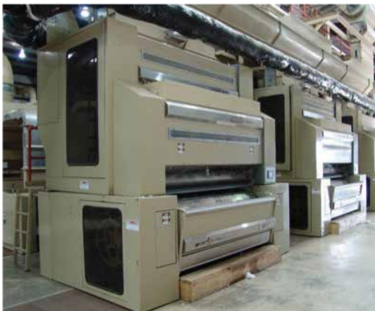
Figure 29. Brush type saw gins
