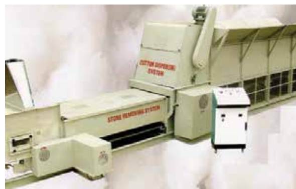
Figure 22. Seed-cotton dispenser with stone remover
