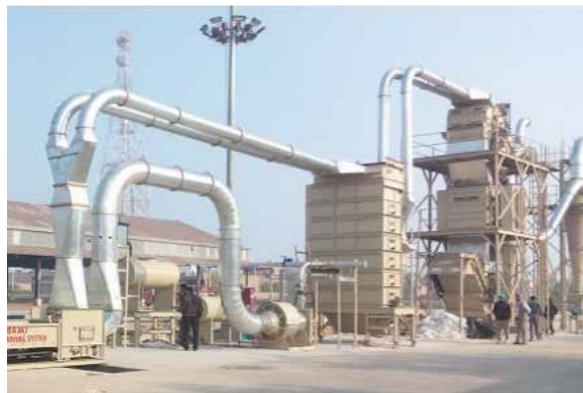
Figure 18. Cleaning & conveying setup for machine picked seed-cotton
