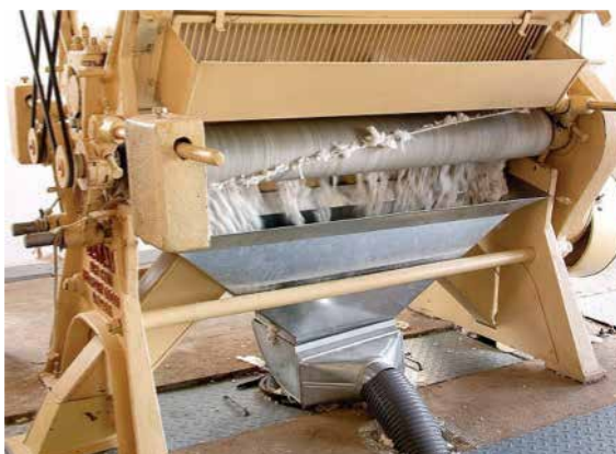
Figure 54. Intermittent lint suction system
