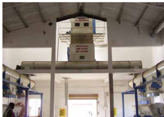
Figure 17. Desired cleaning setup for handpicked seed cotton
