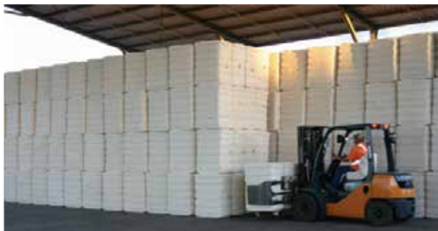
Figure 42. Bale loading by forklift
