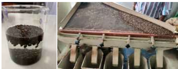
Figure 117. Grading of delinted seeds in water & gravity separation (right)
