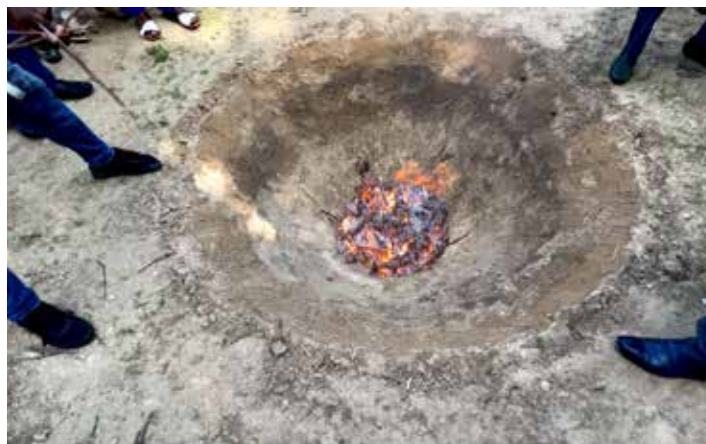
Figure-28. Uppermost stalks of the first layer turn red with a layer of ash around them.
