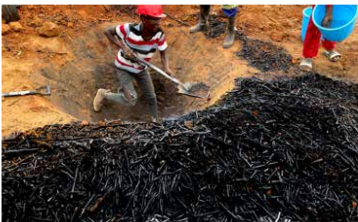
Figure-32. Scooping out biochar after cooling.
