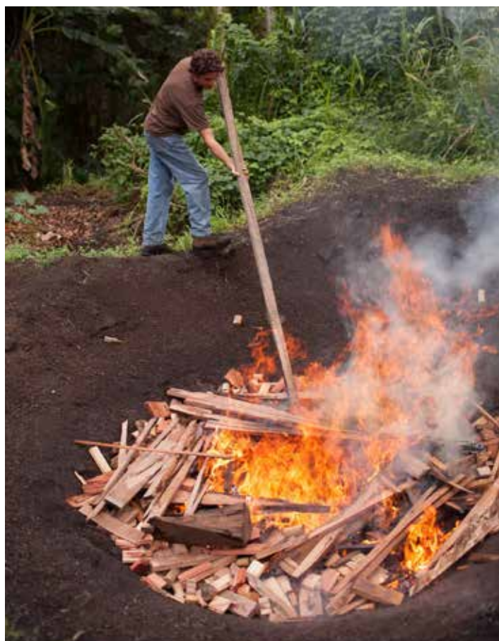
Figure-13. Cone-pit open-earth kiln. Source: https://pacificbiochar.com
