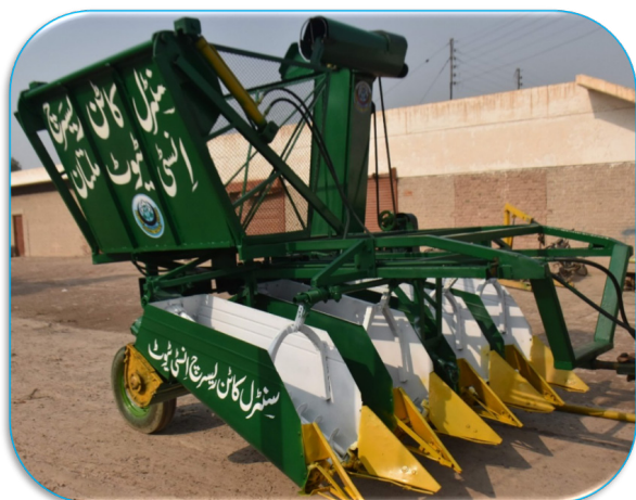
Figure 4. Residual boll picking machine developed by CCRI Multan
