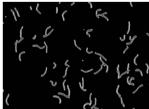
Figure 7 Typical Unprocessed Image Captured by the Cottonscan Instrument
