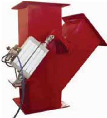
Figure 47. Fire detection and diversion system for ginneries
