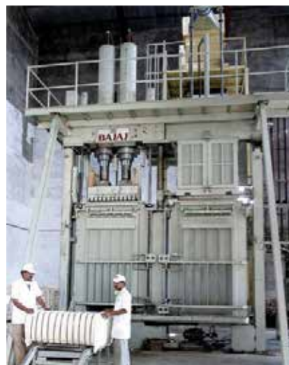
Figure 41. Bales press with bale bagging arrangement
