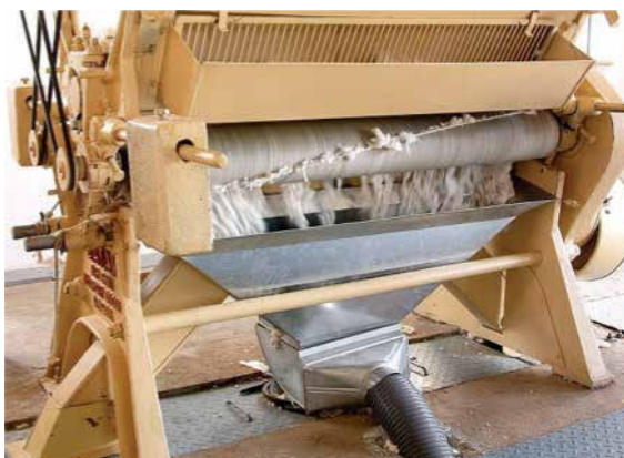
Figure 54. Intermittent lint suction system
