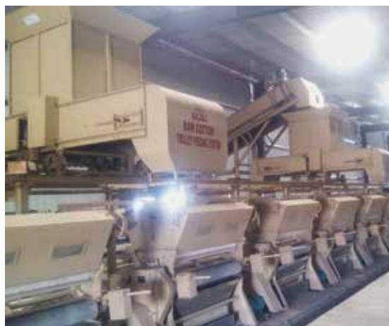
Figure 22. Seed-cotton dispenser with stone remover
