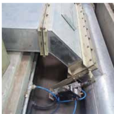
Figure 54. Intermittent lint suction system
