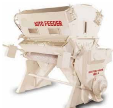
Figure 4. Double roller gin with auto feeder
