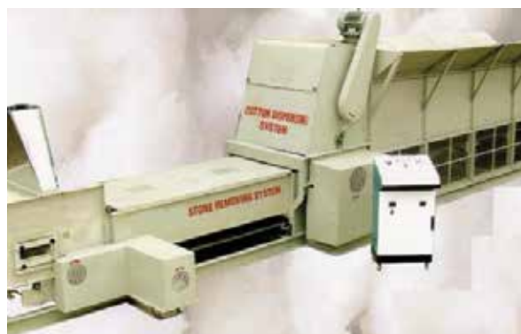
Figure 22. Seed-cotton dispenser with stone remover
