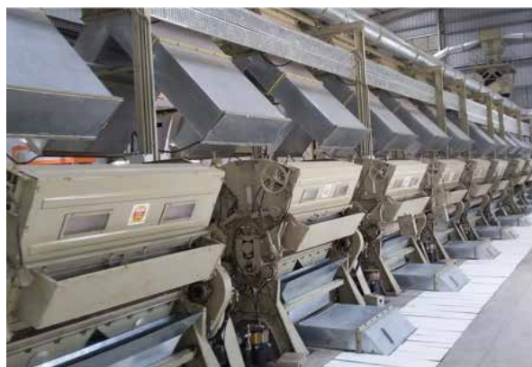
Figure 20. Seed-cotton feeding through central distribution conveyor
