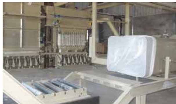
Figure 41. Bales press with bale bagging arrangement
