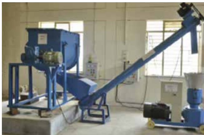
Figure 11. Pelleting plant at the Ginning Training Centre (GTC), Nagpur, India
