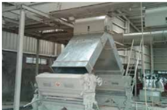
Figure 53. Conventional cotton lint suction system
