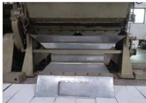
Figure 32. intermittent lint suction system (ILSS)
