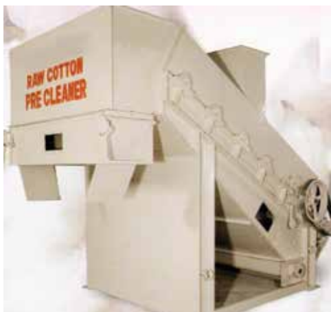
Figure 23. Pre-cleaner for handpicked cotton
