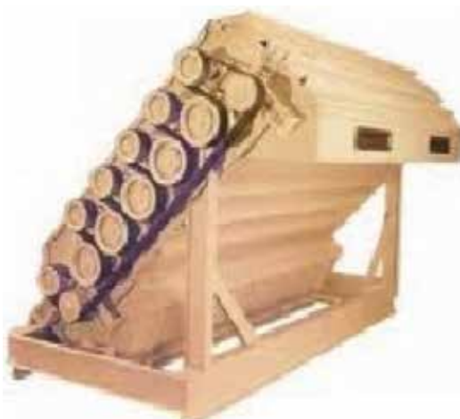
Figure 24. Impact cleaner for leaf trash
