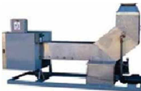
Figure 37. Hot air humidification system used for restoration of lint moisture
