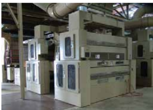
Figure 35. Saw type lint cleaner for machine picked cotton
