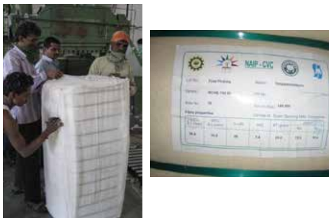
Figure 4. Baling and bale-tagging
