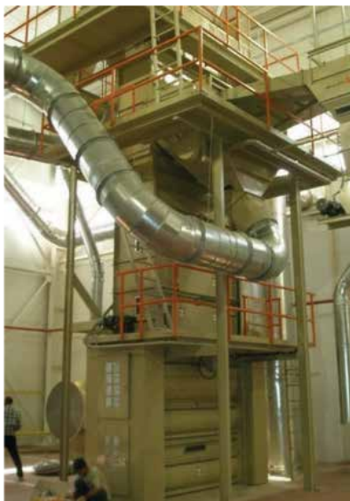
Figure 20. Seed-cotton feeding through central distribution conveyor
