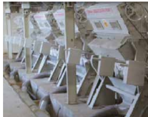
Figure 31. Individual gin lint suction system
