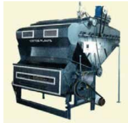
Figure 31. Individual gin lint suction system
