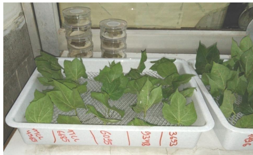
Detached leaf method D: Big Plastic trays- Leaf on aluminum mesh support with 2 ml -2% Sucrose solution
