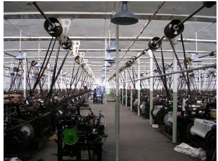
Power transmission by Overhead shafts and belts
