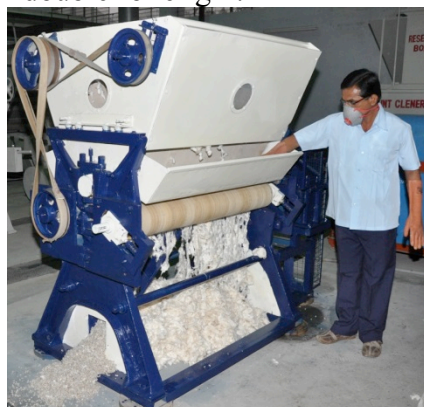
Fig. 8 : Double Roller Gin with self-grooving rubber roller
