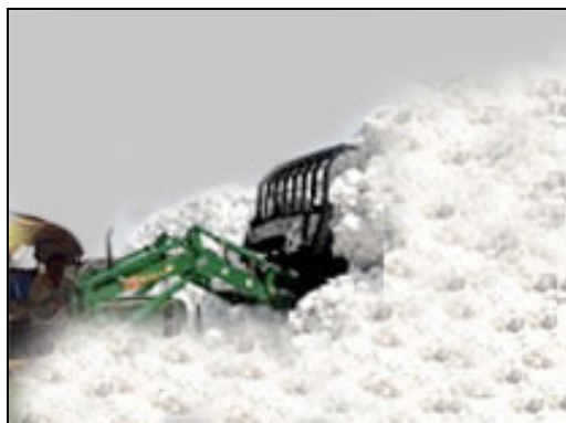
Fig. 2: Tractor Attachment for Heaping of Cotton
