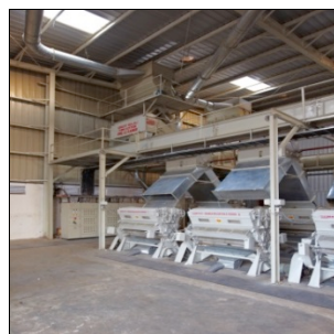
Fig. 6: Twin Auto Regulator Individual Gin Feeding Conveyor System
