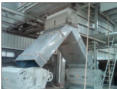
Fig. 6: Twin Auto Regulator Individual Gin Feeding Conveyor System
