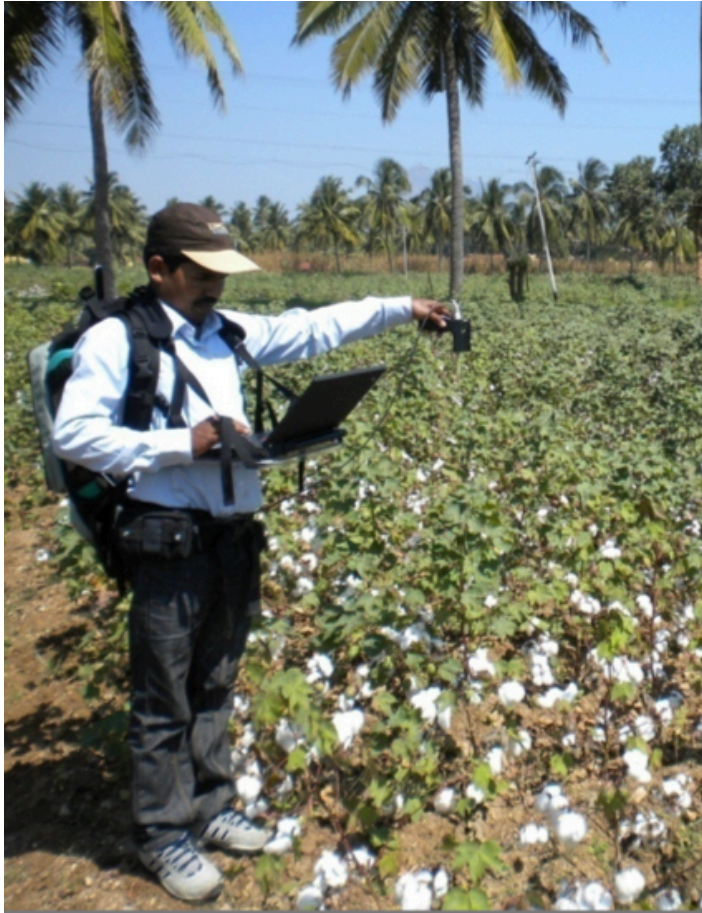
Figure 5. Reflectance measurements of pest infestation using handheld hyperspectral radiometer.
