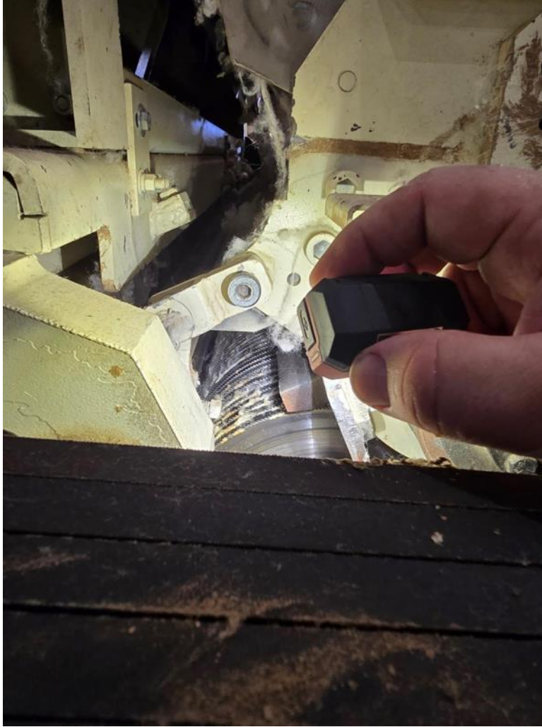
Figure 1 Sticky deposits clogging saws during ginning
