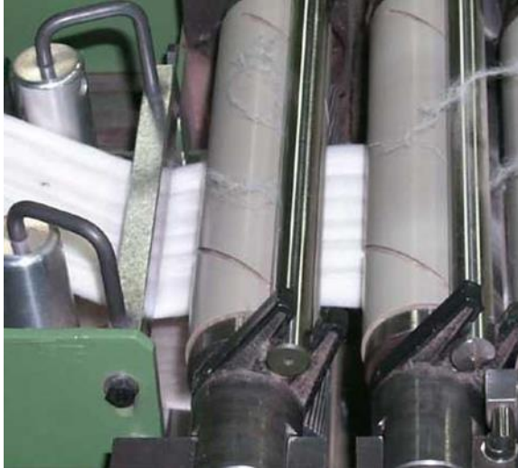
Figure 3 Sticky deposits during drawing
