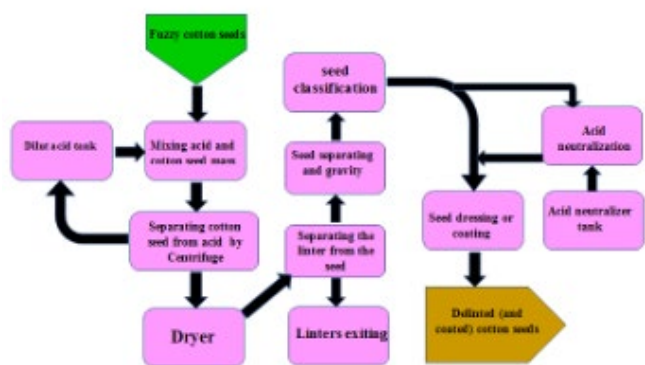
Figure 5. Schematic steps of dilute acid delinting in 4 cotton seed delinting factories in Iran
