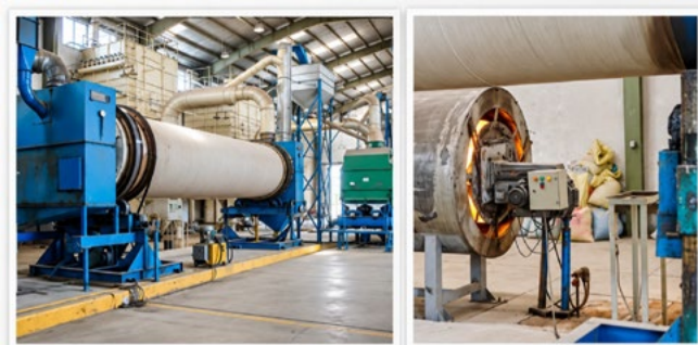
Figure 6 - View of the interior of the Kashmar cotton seed delinting factory, one of four factories located in Iran that works with the dilute sulfuric acid and heat method.
