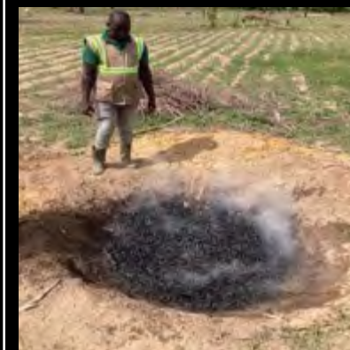
Kon-tiki (open pit) Pyrolysis design
